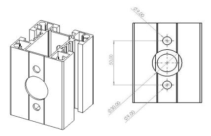
2. Now on the other side drill the holes shown below ensuring that the three centre holes line up with the holes at the front. Ensure that the Dia 3.5 holes go through  $2 \times 10^{-5}$  x wall sections to allow for the 32mm long self-tapping screws.
